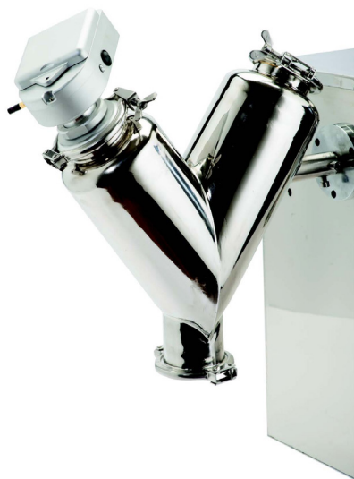
Figure 1. Mounting of the MicroNIR PAT system into the V-cone blender
